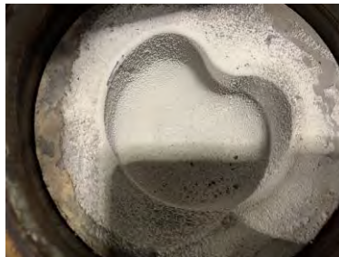
Jenbacher piston with siloxane residue
