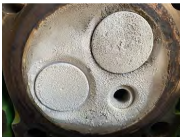
Cylinder head with siloxane residue
