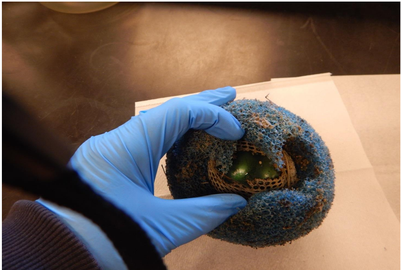
This SmartBall was used to inspect sewer lines for SRSD and was retrieved out of a debris bin by Agency staff on December 17
