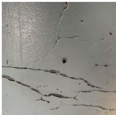
Figure 4: Failed SBS Spill Vault Coating
