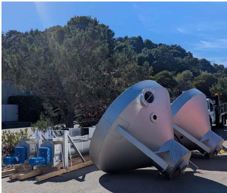
New Huber Coanda Grit Washers Delivered to CMSA in August 2025
