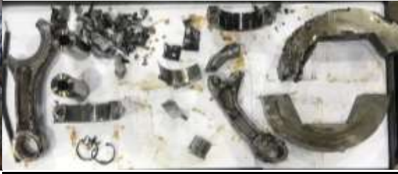
Engine Part Retrieved from Oil Pan
