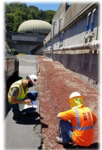
*In-situ soil resistivity testing.*
