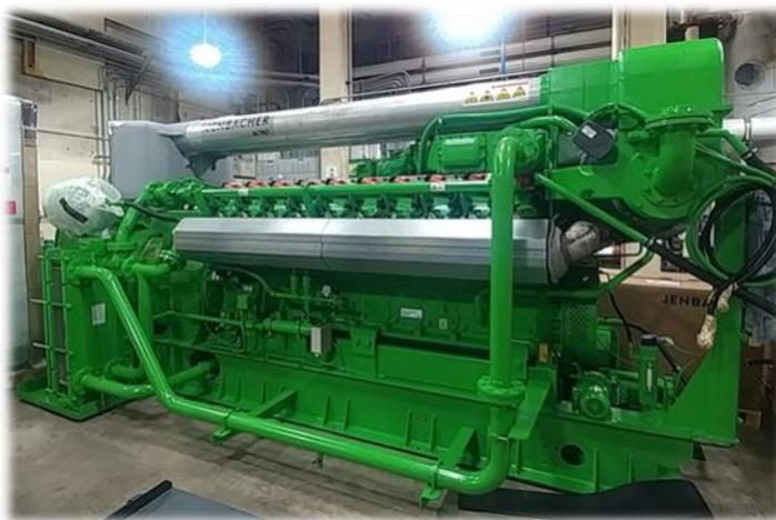
*New Jenbacher cogeneration engine in storage in preparation for installation.*
