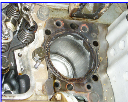
Pictured, left: the cylinder head removed to inspect the piston.
